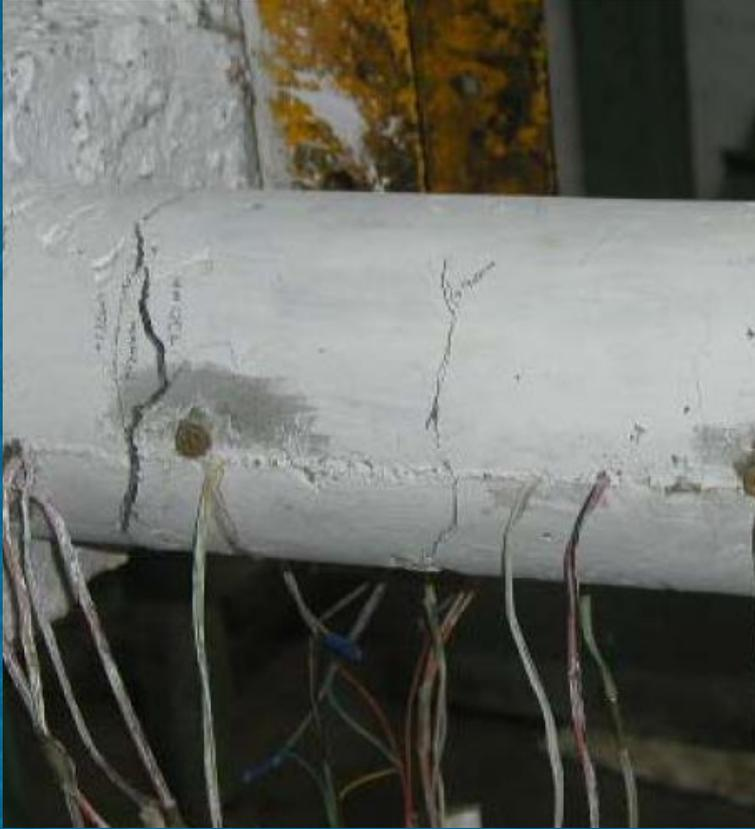
**Tension cracks in Specimen CCYL1**
