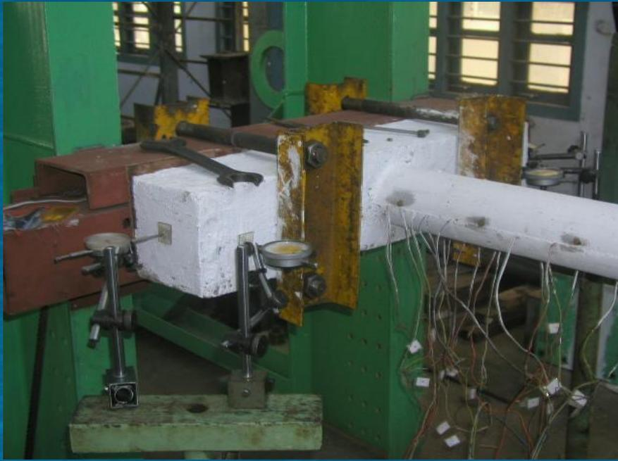
**Fixing the Beam with Channels**
