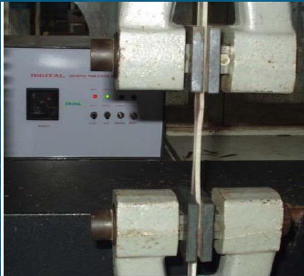
**CAST RESIN TENSION TEST COUPON**
