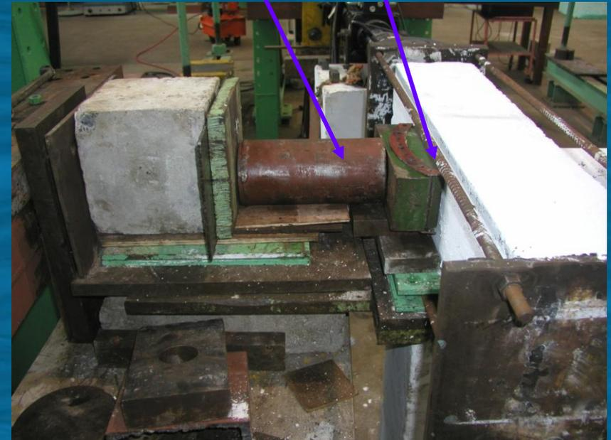
**Jack arrangement for applying axial Load**
