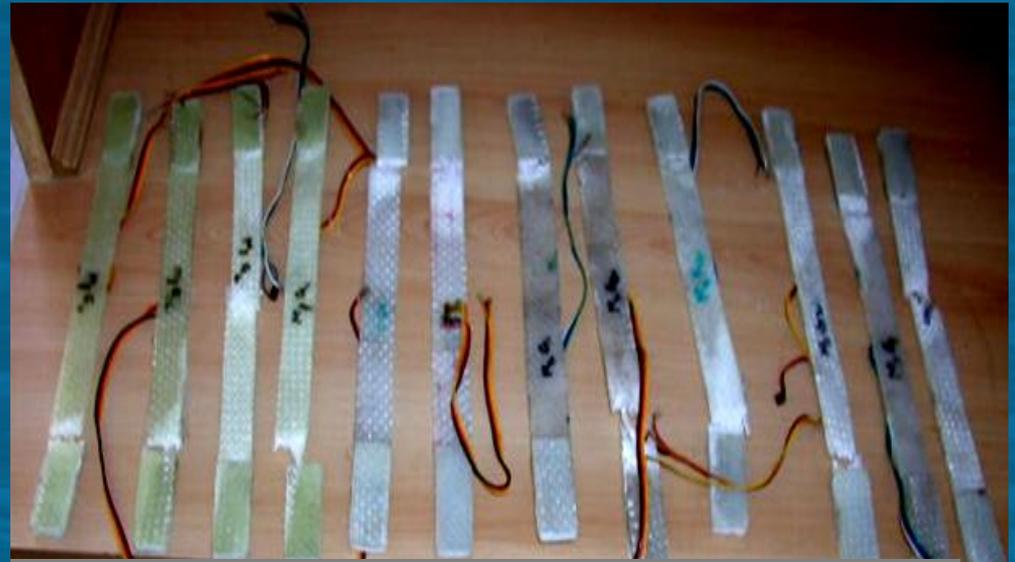
**TENSION TEST COUPONS OF GFRP**
