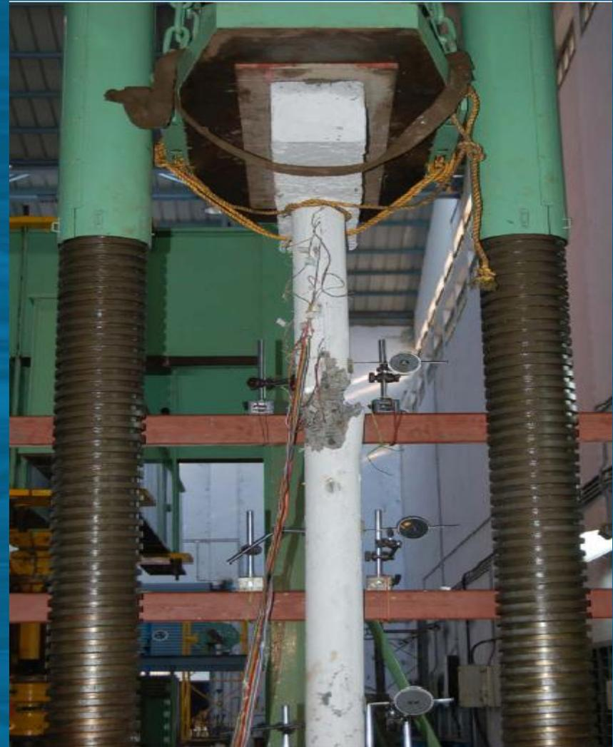
**Failure Mode of Specimen CA1**
