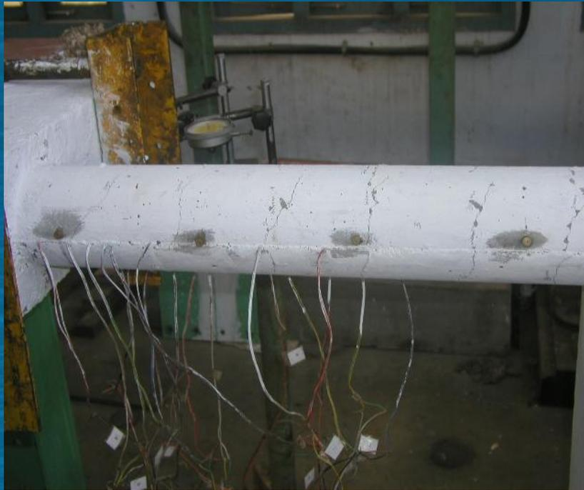
**Formation of Flexural Cracks
