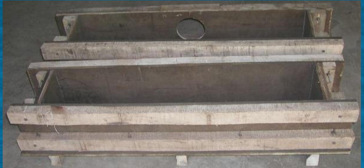
**Wooden Mould used for casting Beams**
