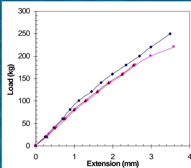
**LOAD/EXTENSION CURVE FOR CAST RESIN IN TENSION**
