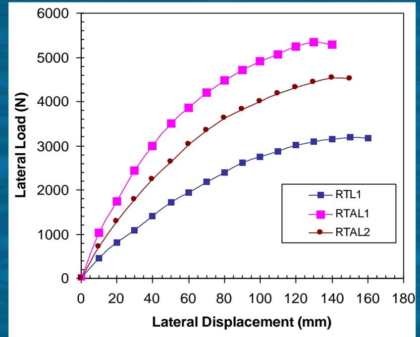
**Lateral Load Vs Lateral Displacement for Retrofitted Specimens**
