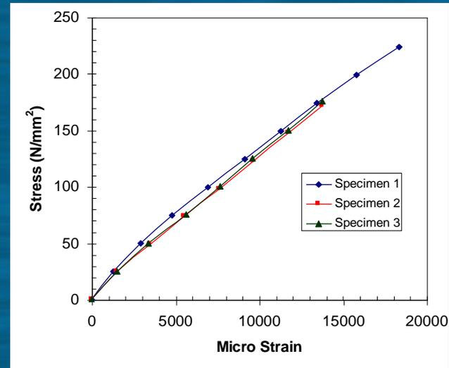
**Stress/Strain Curve for GFRP Composite in Warp and Wept Direction**
