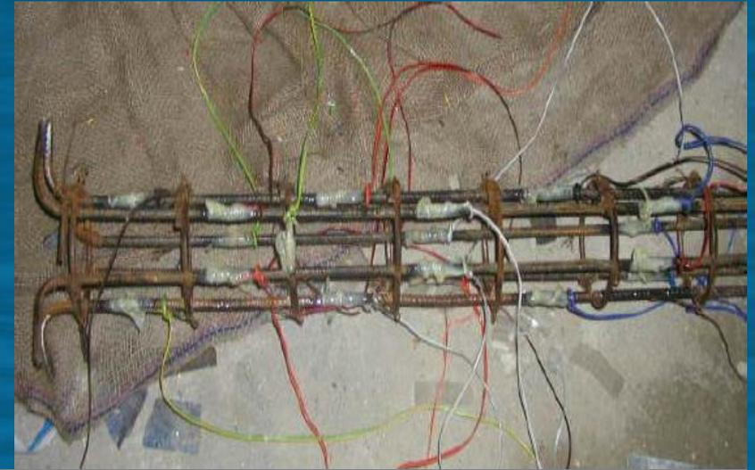
**Water Proofing of Strain Gauges**
