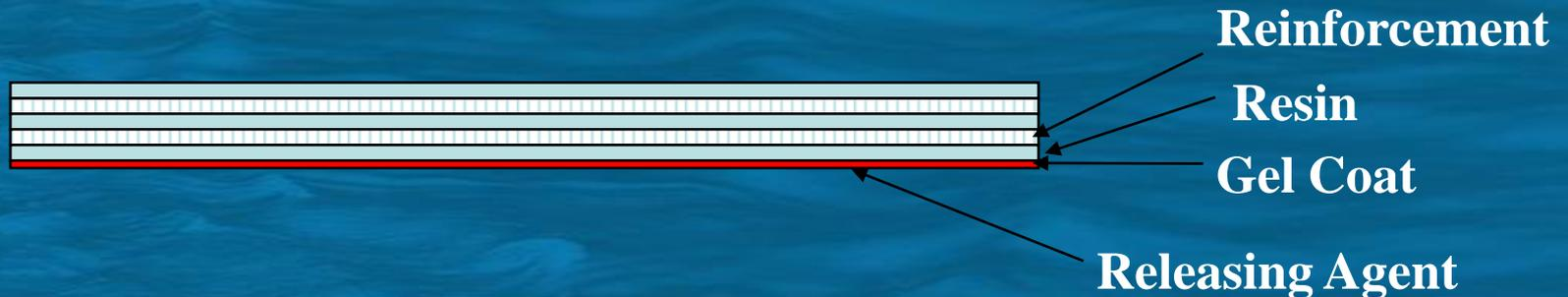
**Structure Through Thickness of Laminate in Hand Lay-up Process**
