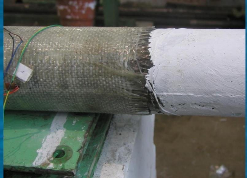
**Cracking of RC Pile Specimen RTAL2**
