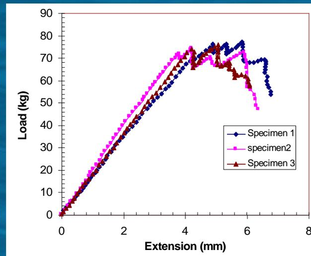
**Load/Deflection Curve for GFRP Composite in Flexure**
