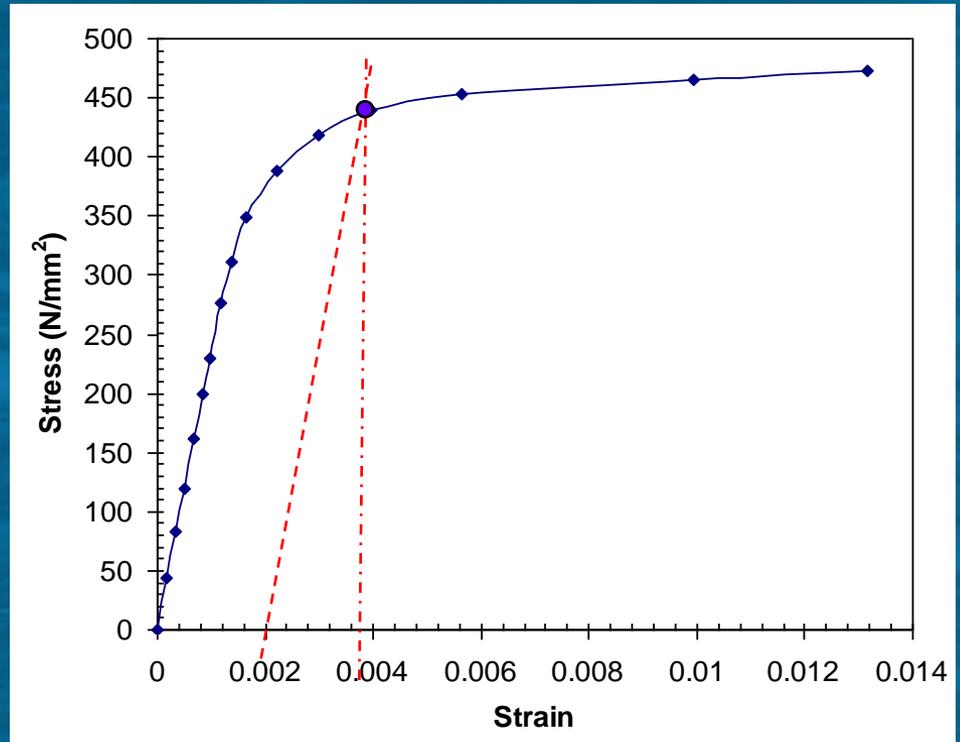
Stress vs Strain curve for 8 mm HYSD steel bar
