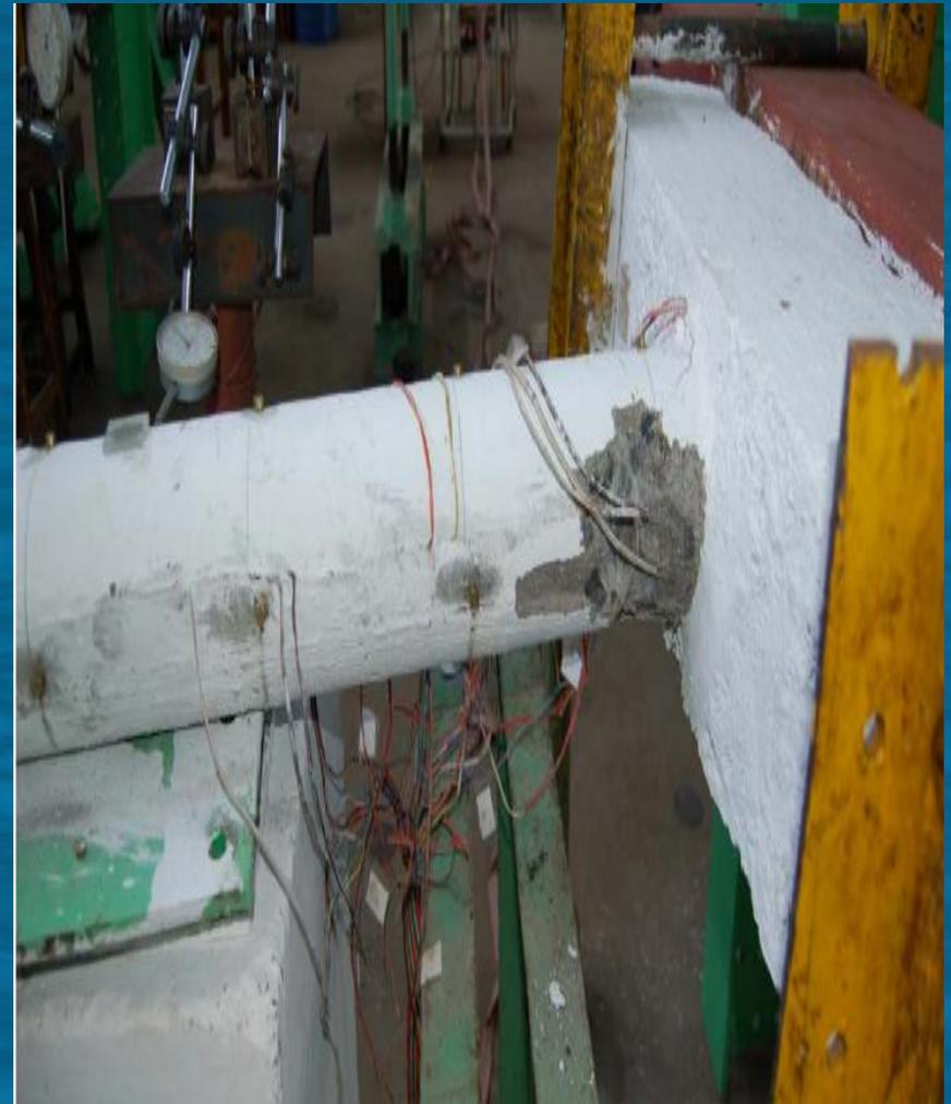
**Failure of concrete in compression for Specimen CL1**
