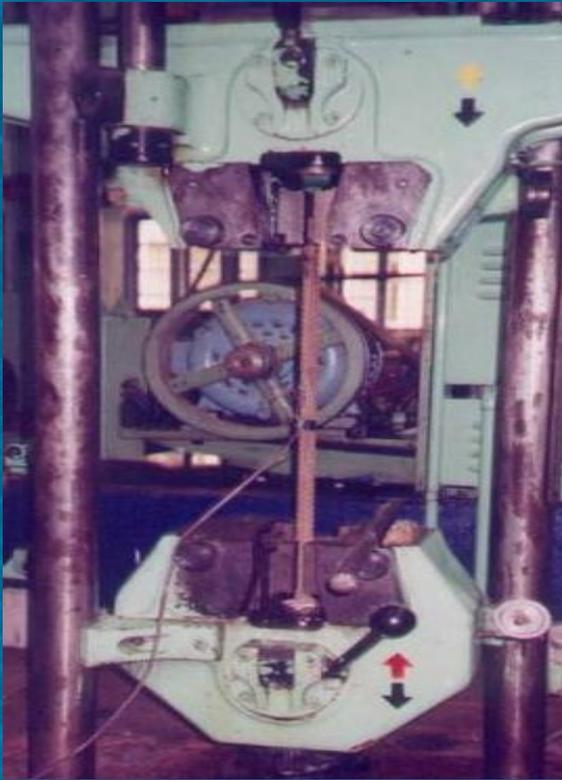
Test Setup for Steel Reinforcement Testing
