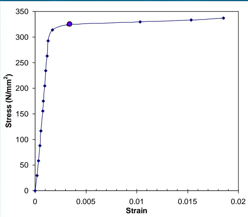
Stress vs Strain curve for 6mm mild steel bar
