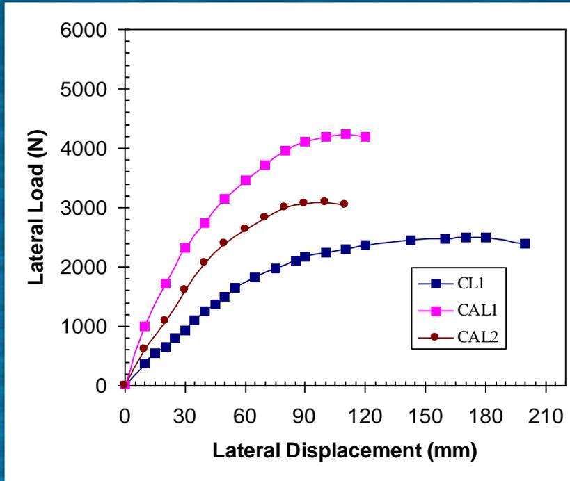
**Lateral Load Vs Lateral Displacement for control Specimens**
