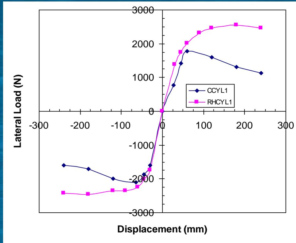
**Stiffness curves for control and rehabilitated specimens**
