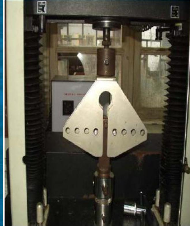
**Flexure Test Set-up**
