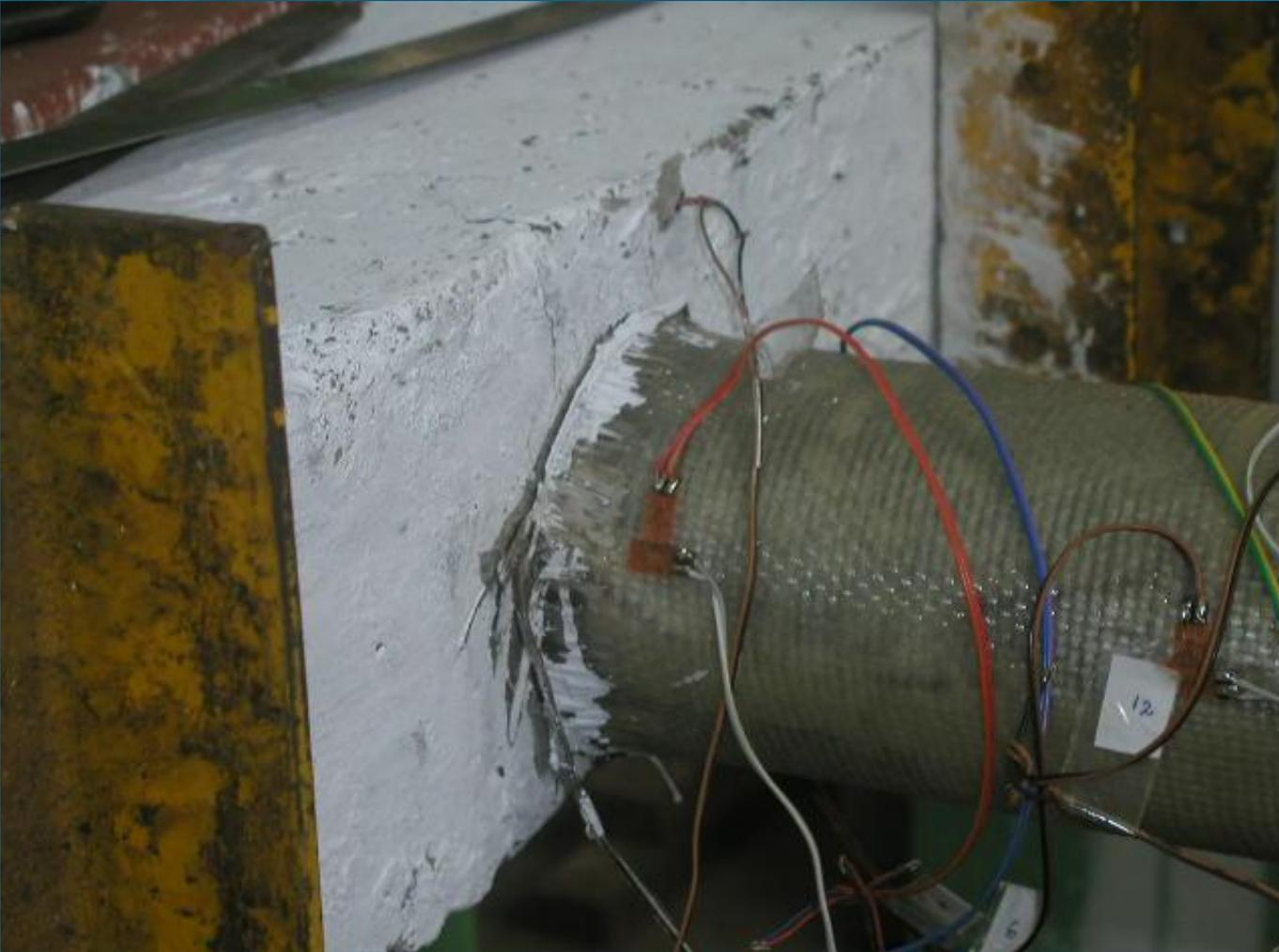
**Failure of Pile Specimen RTCL1**
