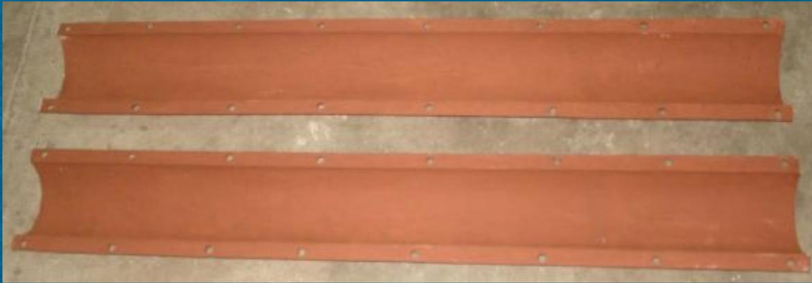
**Steel Mould used for casting Column**
