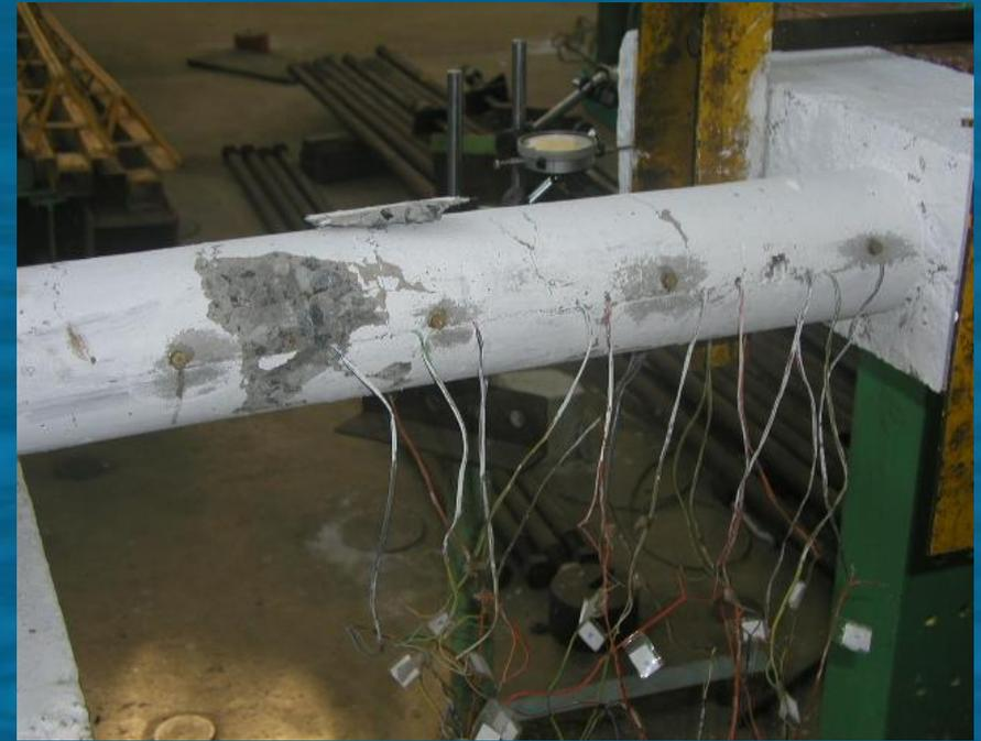
**Crushing Concrete on Compression
