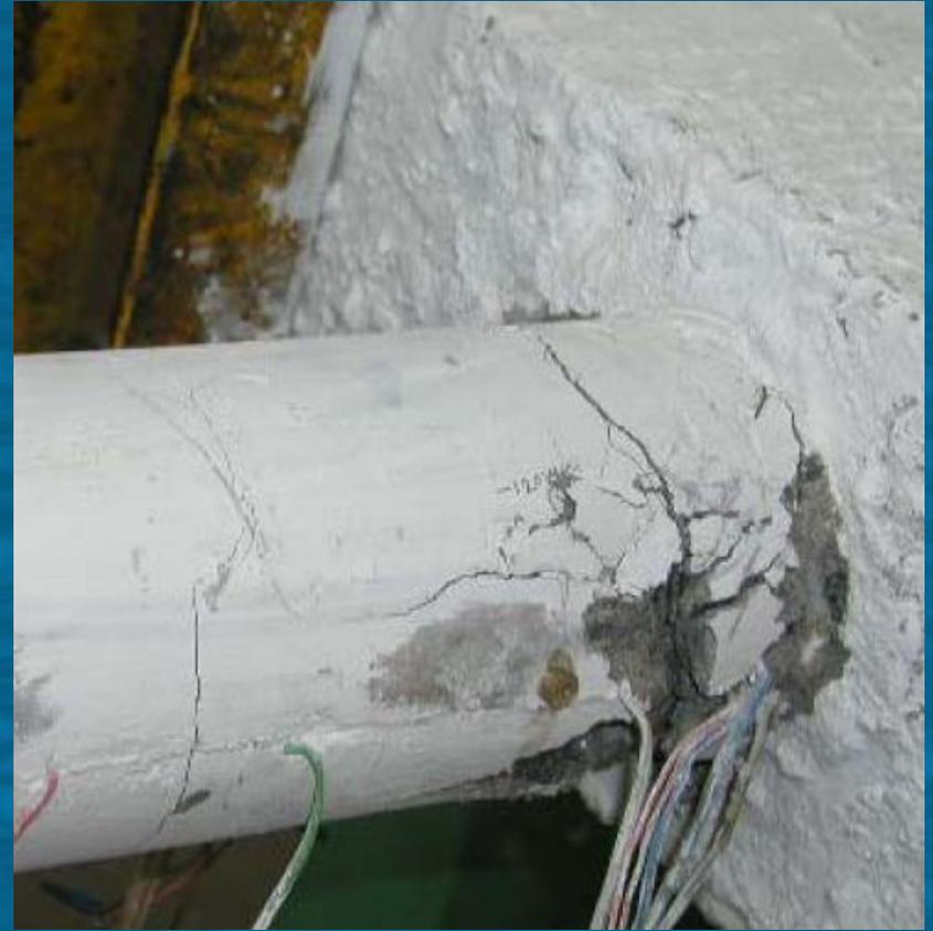
**Crushing of Concrete in Specimen CCYL1**
