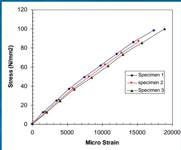
**Stress/Strain Curve for GFRP Composite in 45° Direction**
