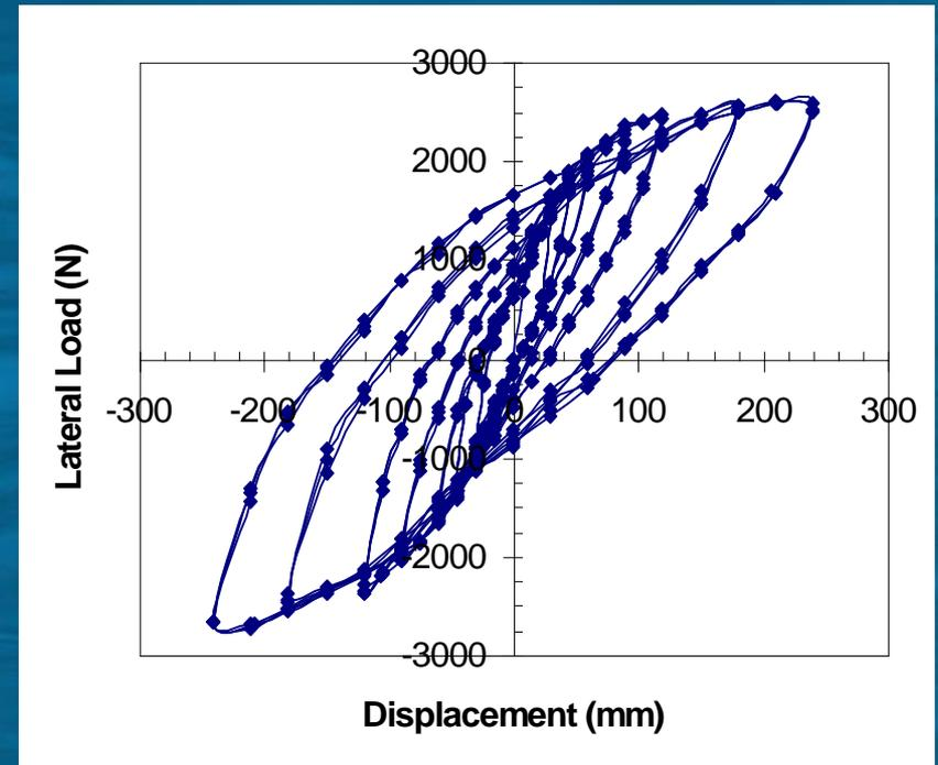
**Hysteretic loops for Control and Rehabilitated Specimens**
