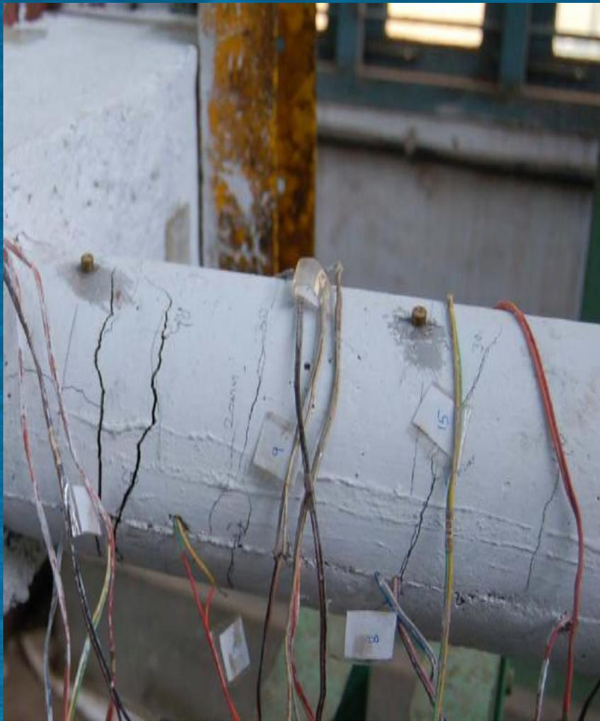
**Failure of Pile in Tension for Specimen CL1**
