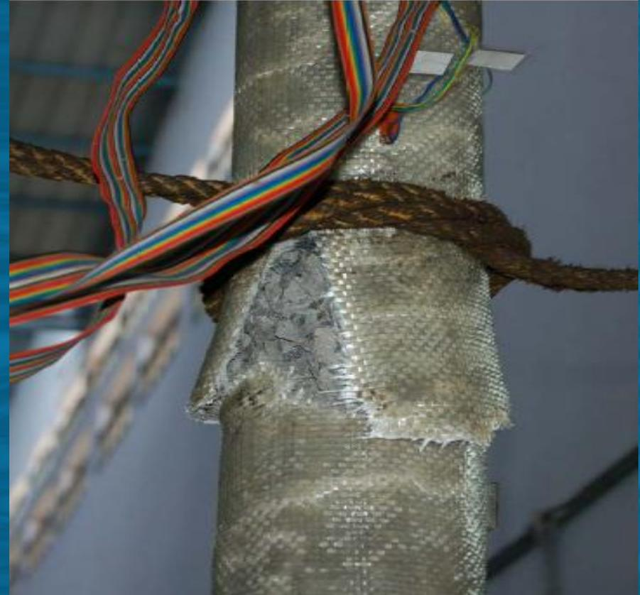
**Failure of GFRP Wrap by Rupture in Specimen RTA1**
